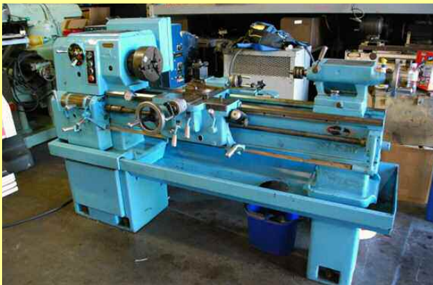
CINCINNATI Engine Lathe with taper attachment 10" 4 jaw chuck and face plate, 12.5" Swing, 36" Centers, Some Tooling ..... $4,500
