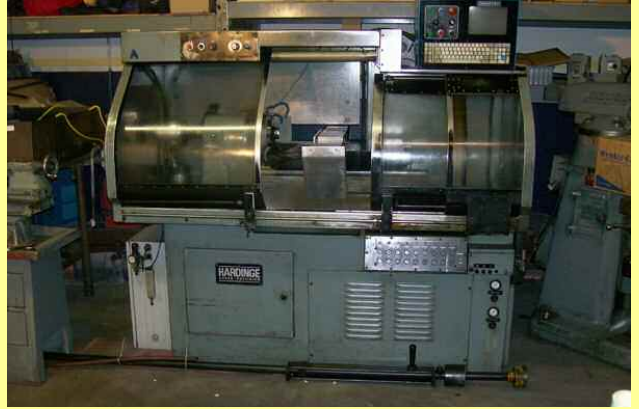
HARDINGE Omniturn CNC Lathe Model AHC New in 1982 – Gang Style Tooling – with Barfeed – New Keyboard – 5 Collet Nose –Extra Parts for Bar Feed and Lathe . $10,000
