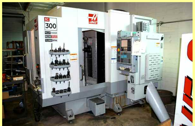
HAAS EC300 4 axis Horizontal Machining Center – New in 2006 – X=20" – Y = 18" – Z=14" – B = 0.001 Positions, 2 pallets, 30 HP motor, Spindle Speed 12,000 rpm, Cat #40, 24 ATC Side Mount Tools . . . . . $115,000
