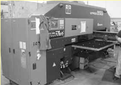
2000 AMADA VIPROS MDL 205050 CNC TURRET PUNCH, FANUC CTRL, 31- STATION, 22 TON, BRUSH TABLE
